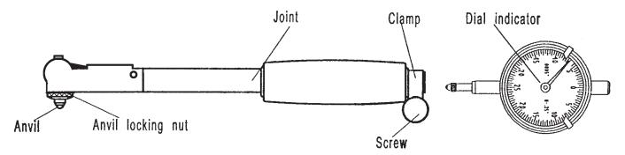
Insert the dial indicator's stem into the bore gage handle and tighten the clamp. The dial gage must be inserted deep enough to "preload" or move the needle about 1 revolution (0.050").
