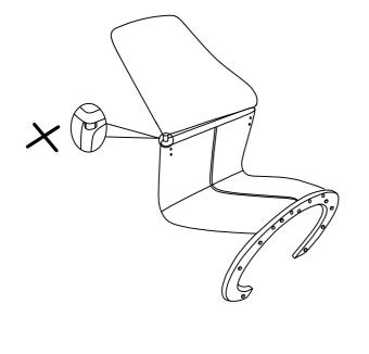
Step 2-a: Place the backrest (B) into the holes on the seat (A). Push down to make sure the screw holes on the backrest (B) are aligned with the screw holes on the seat (A). Screw in all necessary hardware as shown only halfway, do not completely tighten.
