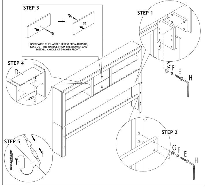
NOTE : MUST TIGHTEN SCREWS PERIODICALLY. WITH USE SCREW MAY BECOME LOOSE. CHECK TIGHTNESS OF ALL SCREWS EVERY 6-8 WEEKS CLEANING INSTRUCTION : AFTER ASSEMBLE, CLEAN & POLISH THE COMPLETED PARTS IF NECESSARY WITH SOFT CLOTH AND INDUSTRIAL RECOGNIZED FURNITURE POLISH.
