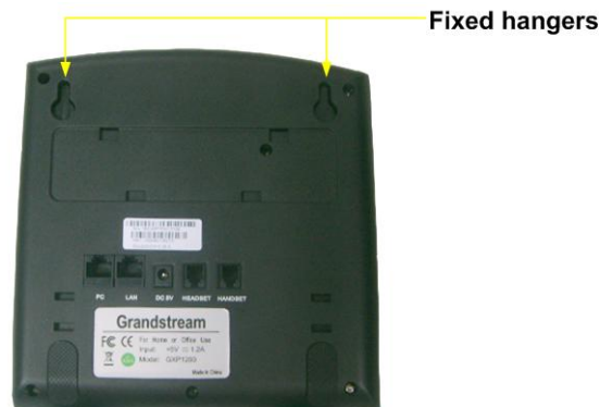
Figure 3: Location of the fixed hangers on GXP-1200
