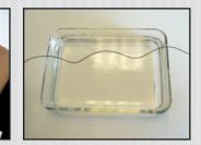
When a trained Nitinol Spring is bent out of shape, and then released into hot water, it turns back to its original shape
