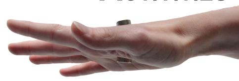
Students can feel the opposing electric force generated by just laying the aluminum ramp flat and holding the NIB magnet in their hand and running their hand across the aluminum.
