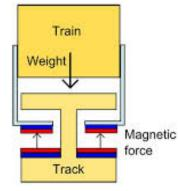
The video explains that trains are built using the principle of magnetic levitation. Note that the train is "floating" on the track and because there is no "friction" the train can go super fast.
