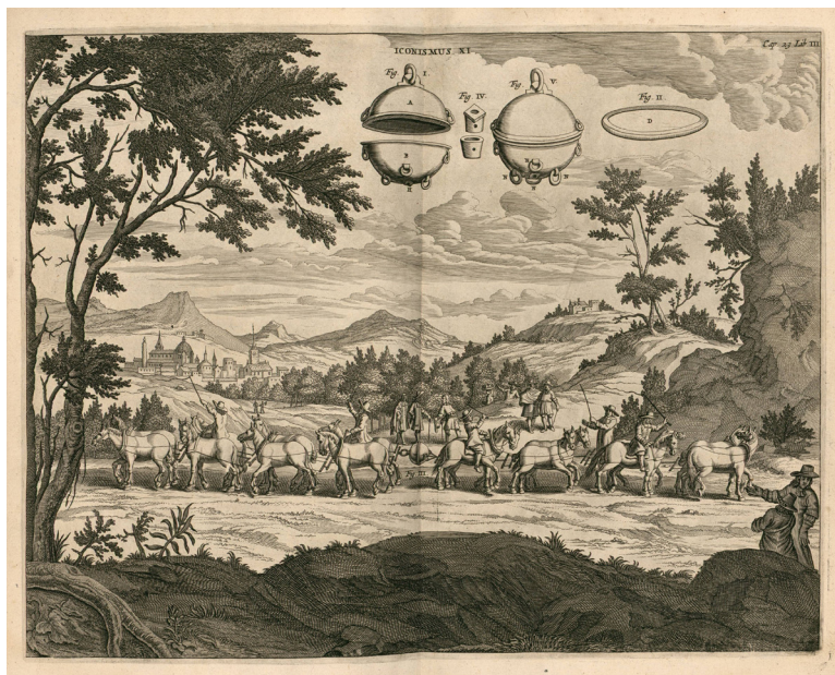
Engraving showing Otto von Guericke's 'Magdeburg hemispheres' experiment - 1672
