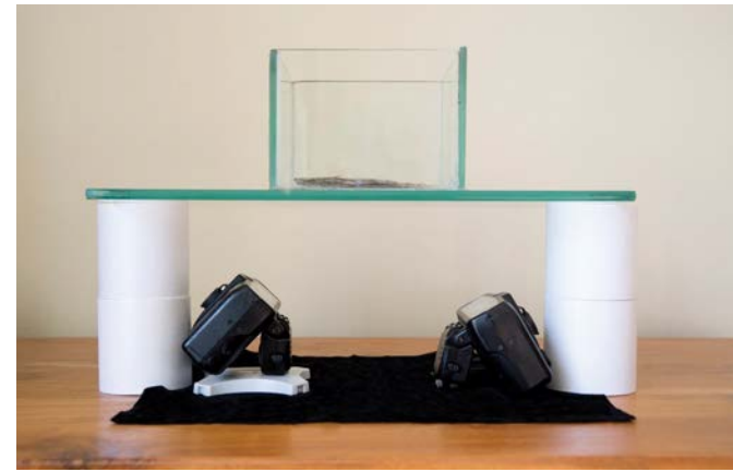
Dark field illumination set-up with subject raised up from the table on a sheet of glass.
