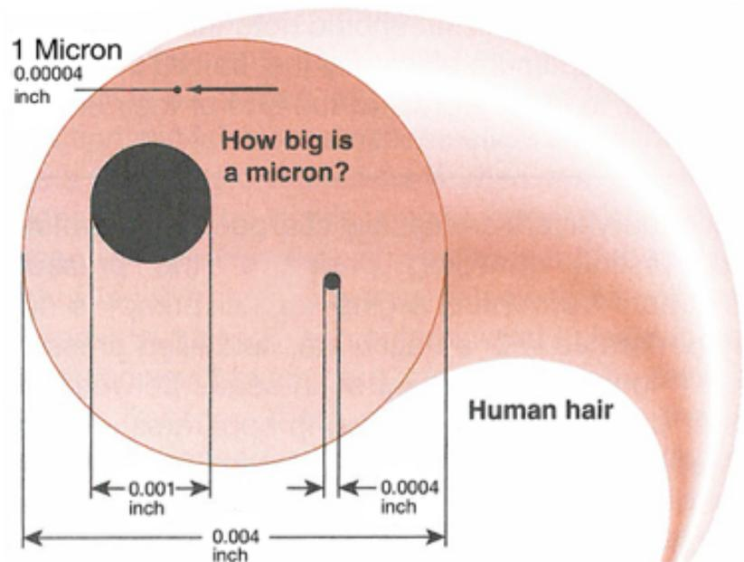
The number one cause of failures on common rail HP pumps and injectors is from contamination in the fuel. Failures of common rail HP pumps and injectors have occurred on initial cranking, engine start up, or on the test drive from contamination entering the fuel system.
