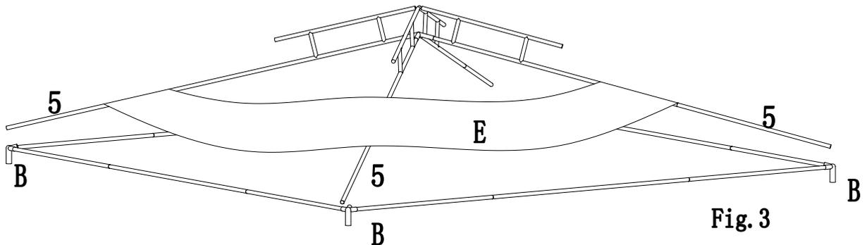
Fig.3: Insert another end of top short pipe (5) into pipe connector (B). Put small canopy (D). (See next step diagram)
