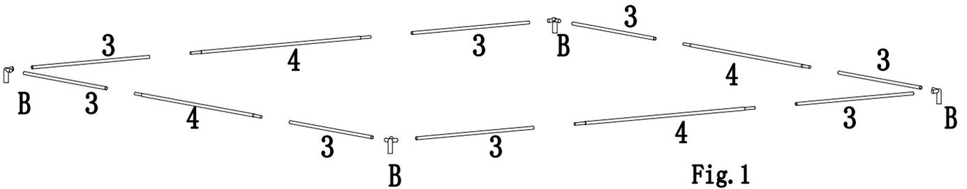
Fig.1: Insert both ends of short support pipe (4) into long support pipe (3), then insert another end of long support pipe (3) into pipe connector (B), with gradient circular tube upwards.
