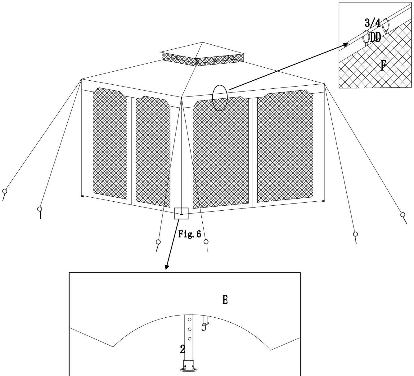
Fig6: At last, unfold the big canopy (E), put hooks of canopy four corners into holes of down posts. Use rope (BB) to tie up four corners, strengthen with big stake (CC). Hang mosquito netting (F) onto support pipes (3,4) with ring (DD).
