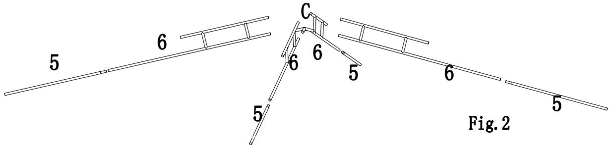
Fig.2: Insert one end with contracted pipe of top short pipe (5) into top long pipe (6), then insert top long pipe (6) into big top connector (C), put big canopy (E) onto frame before installing fourth top long pipe (6), do not spread out. Insert fourth top long pipe (6) into big top connector (C). (See next step diagram)
