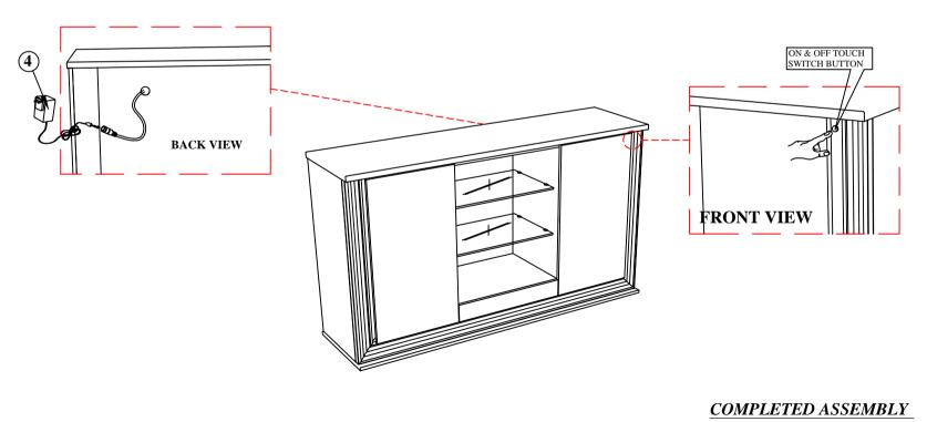
NOTE: MUST TIGHTEN SCREWS PERIODCALLY OR SCREWS WILL BECOME LOOSE.CHECK TIGHTNESS OF ALL SCREWS EVERY 6-8 WEEKS.
