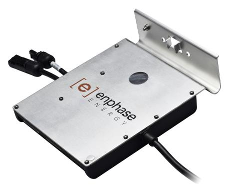
The **Enphase** M215-Z Microinverter delivers increased energy harvest and reduces design and installation complexity with its all-AC approach. With the advanced M215-Z, the DC circuit is isolated and insulated from ground, so no Ground Electrode Conductor (GEC) is required for the microinverter.
