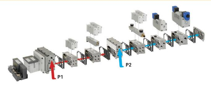
**Pressure Zoning** Multiple Pressure Zones (P1 P2 ... Pn) provide flexibility to meet a variety of applications. Supplying the valves on the manifold with different pressures will allow for variable force output from any attached actuators. In addition, you can control vacuum and remove supply pressure from certain sections while leaving other areas operable. This can be useful in safety applications as well as for maintenance.
