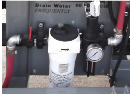
Figure 17: Shut off valve, filter, and regulator for pulse system
