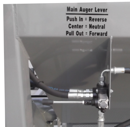
Figure 23: Auger hydraulic motor control lever
