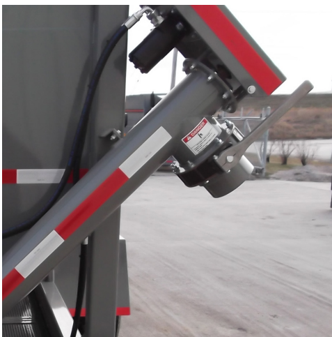
Figure 9: Rear discharge auger butterfly valve lever
