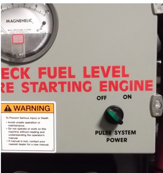
Figure 6: ON/OFF switch for pulse control
