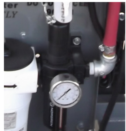
Figure 27: Pulse Air control system- water trap and gauge
