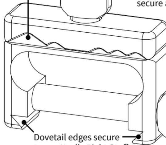
Use clamp knob to secure and release CA-1 from rails and L-plates.
