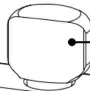
Use pinch bar knob to secure and release cables.
