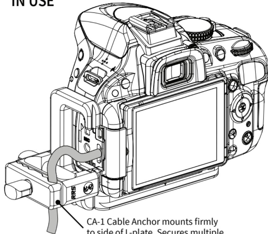
CA-1 Cable Anchor mounts firmly to side of L-plate. Secures multiple cables to prevent accidental release.
