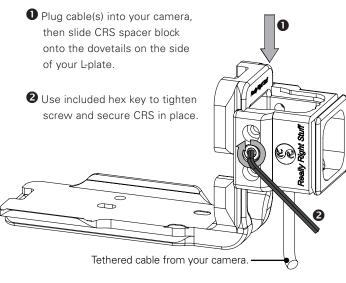
\* For clarity of illustration, Lplate is not shown mounted to camera. In actual use your Lplate will be mounted to your camera. In Step 3 & Step 4, the CRS is shown on end to make it easier to illustrate how the locking bar slides into place.
