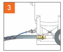
Inlet/outlet to blast machine, Air Prep, etc.
