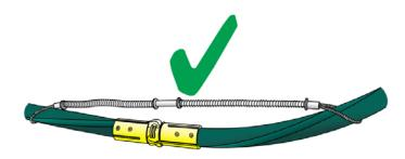
The Whipcheck MUST be fully extended and lay flat along the hose
