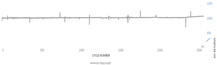
99% round trip efficiency is maintained for over 2300 cycles.
