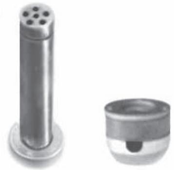
The picture to the right shows the plunger with the groove and bleed holes at the end as well as the port in the barrel.
