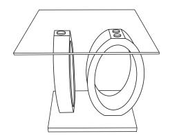
Finally, lean the table with extra care and tighten the bolt.(E&F).
