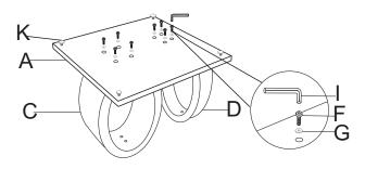
Firstly, fix the table leg with table base but do not fully tighten the bolt(F).
