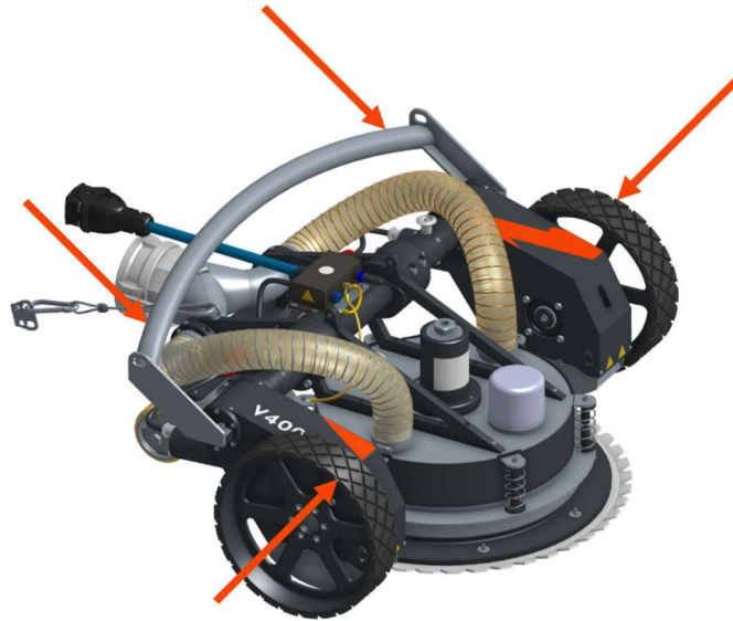
Holding points suitable for robot handling.
