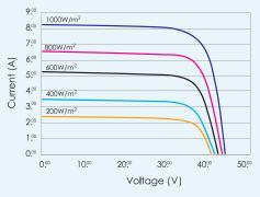
Average efficiency reduction of 4.5% at 200W/m<sup>2</sup> according to EN 60904-1.
