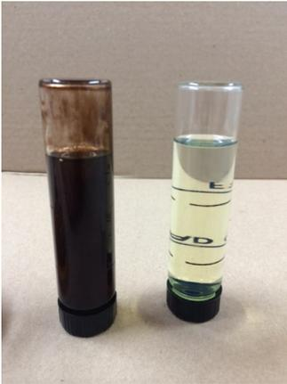
The picture on the left shows two vials of diesel fuel where sulfuric acid has been added. In the vial on the left Stanadyne Performance Formula has been added while DieselBOOST Diesel Fuel Upgrade has been added to the vial on the right.
