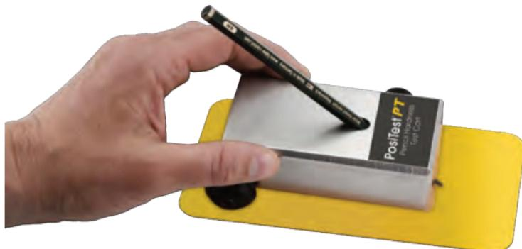
3. If required, continue to perform the test, moving down the hardness scale with each test, until a pencil will not scratch or deface the coating. This pencil is reported as the scratch hardness.
