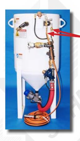
**Step 1 Start** by removing the Twinline hose assembly from the existing vessel.
