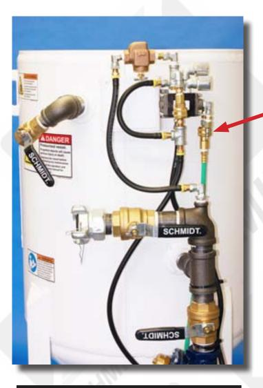
Step 14 Attach orange hose and black hose to the quick-connect fittings on the front Control Valve.
