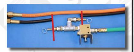
Step 11 Cut Twinline black hose as shown, creating a gap large enough to fit valve assembly into the gap.
