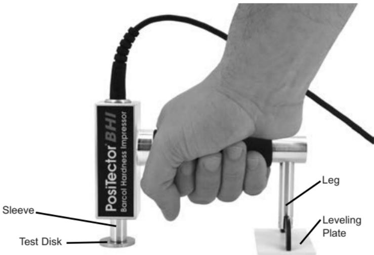
Verify accuracy at the beginning and the end of each work shift. During the work shift, if the Gage is dropped or suspected of giving erroneous readings, its accuracy should be re-verified.
