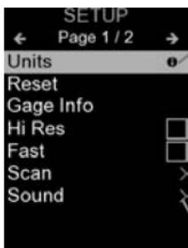
When a Menu option is highlighted, the icon indicates on-gage help is available. Press or touch the icon to display the help. A formatted PDF containing all on-gage help items is available at [www.defelsko.com/help](http://www.defelsko.com/help)
