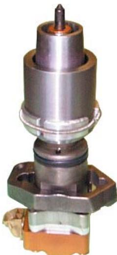
Quickly push the driver down the guide, until the seal ring drops into the correct slot. The end of the driver will expand to match the contour of the guide. (Left Picture)
