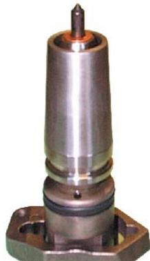
Place the guide completely over the tip end of the injector. It will provide a smooth continuous surface leading to the center seal ring slot. (Left Picture)
