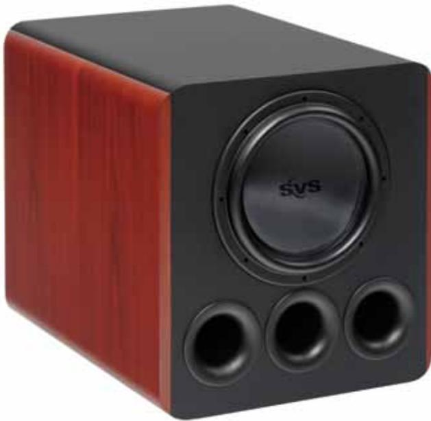
The \$1,139 PB-12 Plus is a classic “big box” subwoofer, measuring 25 inches deep, 19 inches wide, and 21 inches high, and weighing 127 pounds. It features an overbuilt 12 1/2-inch woofer with a fiberglass/pulp composite cone, driven by a switching-type BASH amplifier rated at 525 watts continuous power. The woofer vents through three 3-inch ports that run all the way to the back of the enclosure (which, by the way, is available in gloss black, rosenut, and oak finishes).
