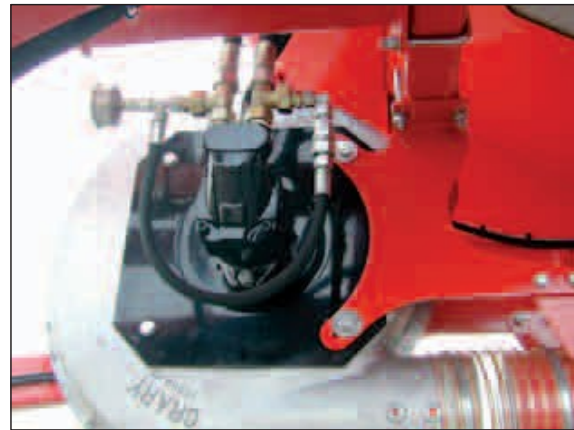
Fan with direct drive
