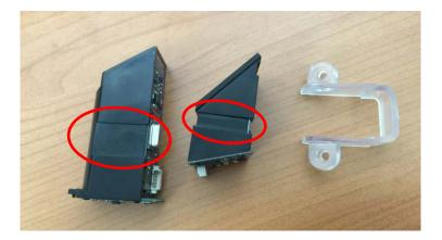
Mount the module beneath the upper part of a case using the bracket
