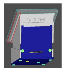
Both module and module cover need to be supported.
